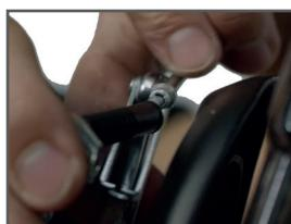
After inserting the front wheel, the brake cable must be hooked in. To do this, press the two brake arms (3) together and place the guide tube (7) in the groove provided for it (as shown). If this is not possible even under great exertion, you can loosen the anchor nut (2) a little and thus extend the brake cable pull (retighten anchor nut (4)).
