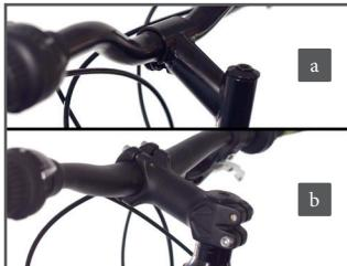
For packing reasons the handlebars were twisted and disassembled. The components must be realigned accordingly by loosening the necessary screws. For Bergsteiger bicycles both cone stems (pages 14-15), as well as A-head stems (pages 16-17) are used.
