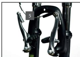
Loosen the outer axle nuts (4) and turn them outwards as far as possible. Unhook the brake cable (5). The brake shoes swivel outwards.
