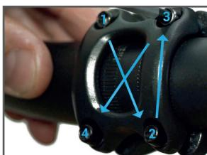
To mount the handlebars to the stem (1), remove the four clamping screws of the stem clamp (3) completely, insert the handlebars, select the correct inclination of the handlebars and carefully tighten the four screws crosswise again.
