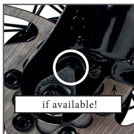
Loosen the two outer axle nuts (2). Push the front wheel into the fork (1).
