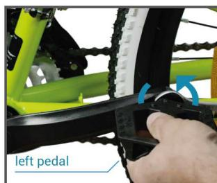
**!** Before each ride, check that the pedals are firmly secured. Especially after the first kilometers you have to retighten the pedals! Loose pedals can cause injury and damage the pedal thread. Damage caused by improper installation is excluded from any warranty.
