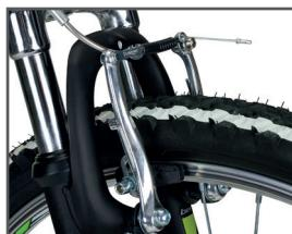
After assembly, both brake shoes (5) must be aligned on the rim and the brake arms (3) must be parallel to each other.
