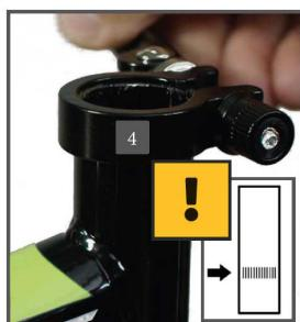
Open the quick release fastener (4). Push the saddle (1) with the seat post into the seat tube (5). Tighten the saddle clamp screw again (alternatively close the quick-release fastener).
