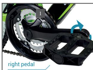
Screw the right pedal on the sprocket side (1) into the crank in a clockwise direction (like a conventional screw).
