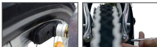
The V-brake is already correctly adjusted at the factory. If it still grinds or the distance between the two brake shoes and the rim is not the same, first make sure that the brake shoes are correctly aligned with the rim. Then the distance can be balanced.
