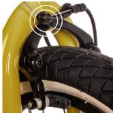
If your bike is equipped with a U-brake, you can loosen the fastening screw of the Bowden cable on the brake arm before mounting the front wheel. With the front wheel in place, squeeze the brake arms together until the brake shoes just clear the rim (about a dime should fit between them) and retighten the bolt.
