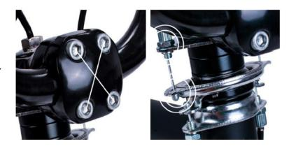
After attaching the handlebars, screw the Bowden cables into the first rotor plate. Then the end of the Bowden cable can be hooked into the second rotor plate. You can pull the second rotor plate up a little. The brake can be adjusted using the adjusting screws on the brake handle and rotor plate.
