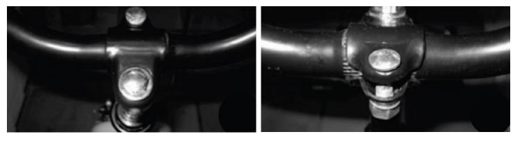
The height and the angle of the handlebar can be adjusted by loosening the steering head screw (picture 1). If you loosen the clamping screw (image 2), you have the option of adjusting the incline of the handlebars to the needs of the child.
