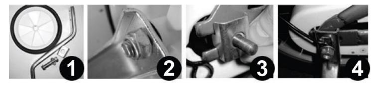
Take the long bolt and slide it through the tire. Put the washer over it, then the jockey wheel retaining iron and screw everything tight with the nut (picture 2). Do the same with the other jockey wheel. Now remove the cap nuts on the axle of the rear wheel. Put the metal lock onto the axle (picture 3). Now you can tighten the jockey wheel again with the axle nut. **The support wheels should sit firmly on the axle**.
