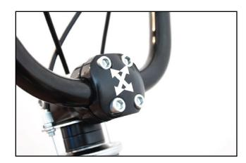
Inserting the Bowden cable for the rear wheel brake is different on a Freestyle BMX than on conventional bikes. After attaching the handlebars, screw the Bowden cables into the first rotor plate. Then the end of the Bowden cable can be hooked into the second rotor plate. You can pull the second rotor plate up a little. The brake can be adjusted using the adjusting screws on the brake handle and rotor plate.
