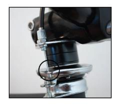
Place the seat tube in the saddle. Put the seat clamp over the frame tube (if not pre-assembled) and insert the seat post.
