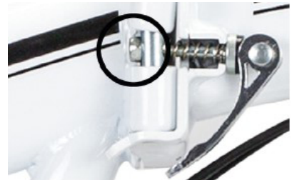
1c) Turn the quick release to the right and fold it over. If this is not possible / too difficult, loosen the opposite nut a little.
