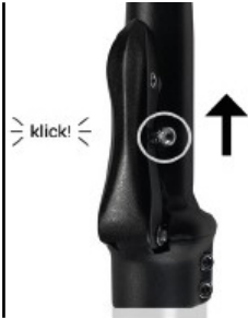
2) Fold the handlebars. The handlebar can be fixed using the folding lever. As soon as you hear the "click" sound, the stem is locked. To fold the handlebars again, slide the latch up and open the folding lever.
