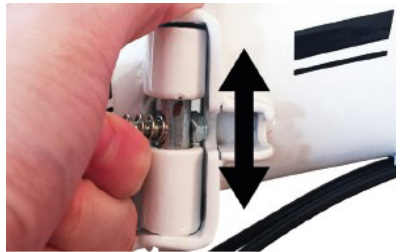
1b) When folding, you should hear a clicking sound. The quick release is now engaged. To unfold later, pull the quick release upwards.
