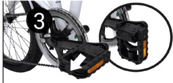
3) Flip pedals. To unfold it, you only have to fold it upwards until you hear a clear clicking sound. To fold, pull the pedals outwards and fold them down.
